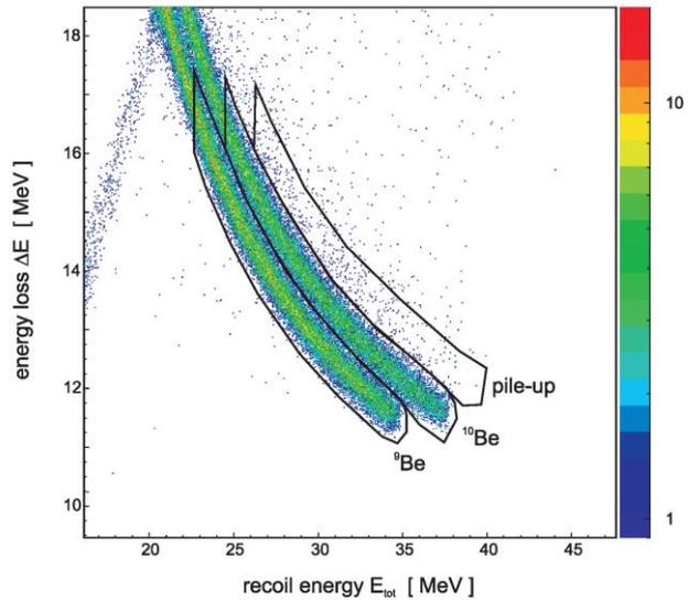
Figure 1. ERD measurement of  $^9\text{Be}$  and  $^{10}\text{Be}$ . Shown is the energy loss versus the total energy of both  $^9\text{Be}$  and  $^{10}\text{Be}$ . Indicated are the regions of interest as well as the region which we took for the pile-up correction.
