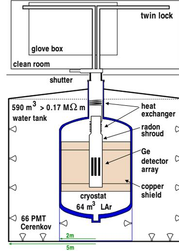
Figure 1: Schematic drawing of the experiment.
