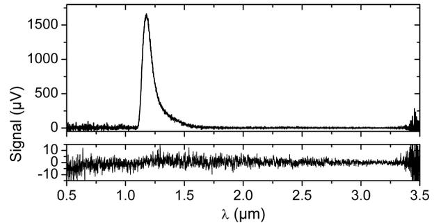
Figure 2: The electron-beam induced infrared emission of liquid argon doped with 10 ppm xenon is shown in the upper panel. For comparison pure liquid argon shows no infrared emission (lower panel).
