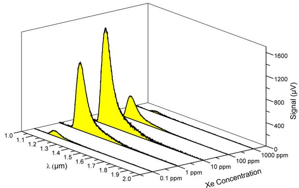
Figure 3: The electron-beam induced infrared emission of xenon doped liquid argon is shown for different xenon concentrations. The broadband emission peaks at  $1.18 \mu\text{m}$ , has an asymmetric shape and a half width of approximately  $0.1 \mu\text{m}$ .
