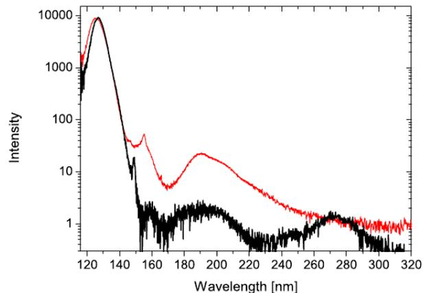
Figure 1: The emission spectrum of electron-beam excited gaseous (red) and liquid (black) argon is shown.
