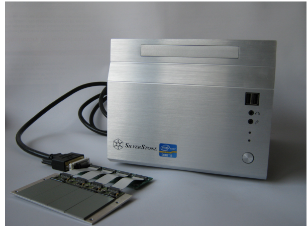
Figure 1: Detector system based on the RadEye1 imager which allows parallel read-out of up to 4 sensor elements.
